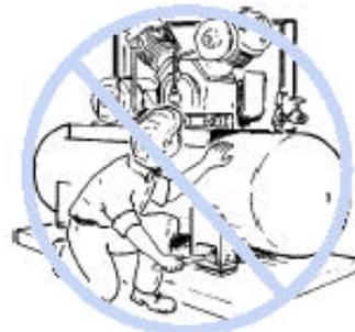
**DO NOT TEST WITH AIR OR COMPRESSED GAS.**
