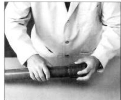
Note: For pipe sizes 6" and larger, two people will be required, a mechanical forcing device should be used, and the joint should be held together for up to 3 minutes.
